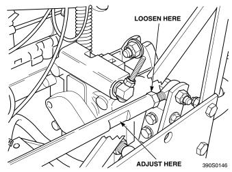
Figure 6-4. LH Steering Control Rod Adjustment
